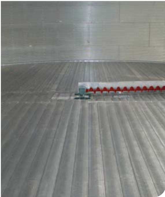
Full perforated plank floors allow for drying or conditioning air to distribute evenly up through the stored product.
