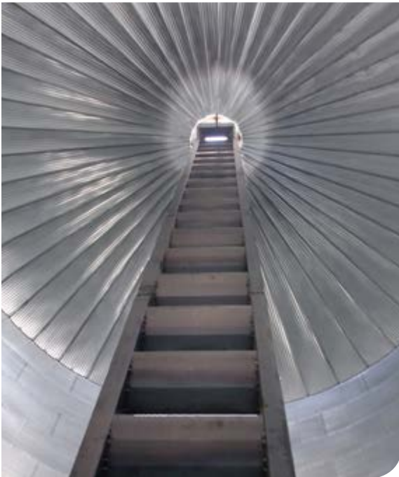
Let-down ladders reduce stress created by flowing materials and help prevent waste from product breakage.
